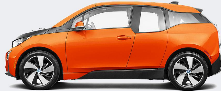
Extended Range Electric Vehicle EREV Example: BMW i3
